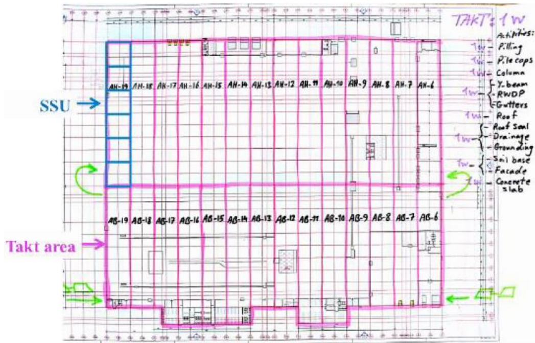
Figure 12. An example of the division of a functional area into takt areas and SSUs. (Dlouhy et al. 2016)
