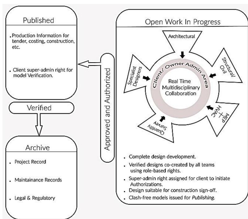
**Figure 6.** Proposed common data environment (CDE) with an open work in progress (OWIP).
