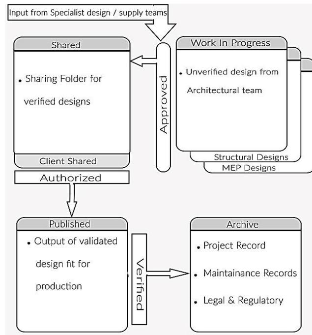
**Figure 1.** Schematics of a common data environment based on PAS 1192-2 (Source: [2]).
